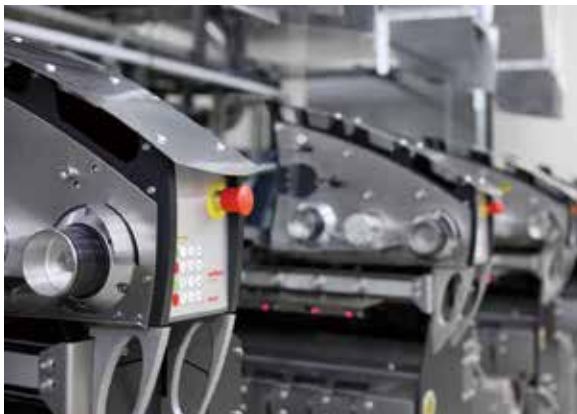
A new driver unit for Wings POY further reduces energy consumption in the winder section by 3%
